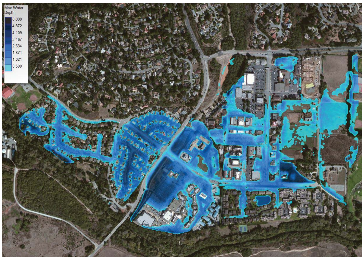
Figure 4-2 Maximum interior drainage water for the 100-year design storm
