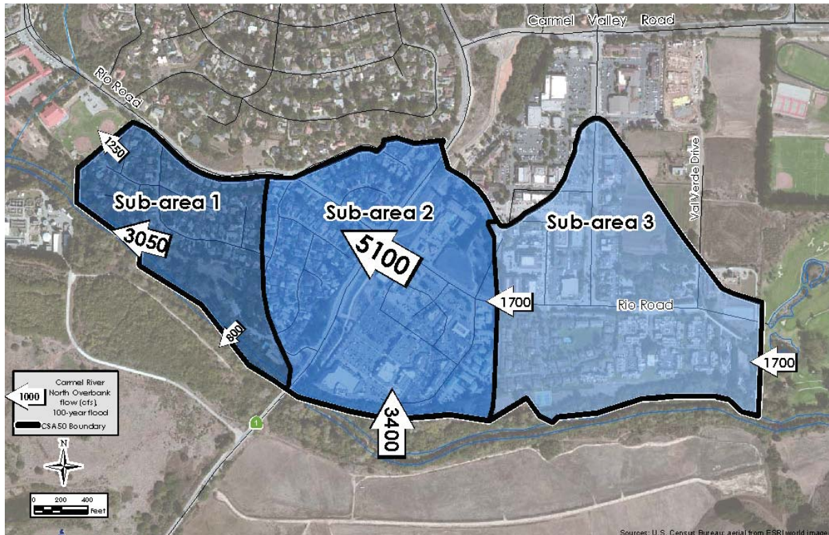
Figure 2-4 Generalized flood hazard sub-areas within CSA-50
