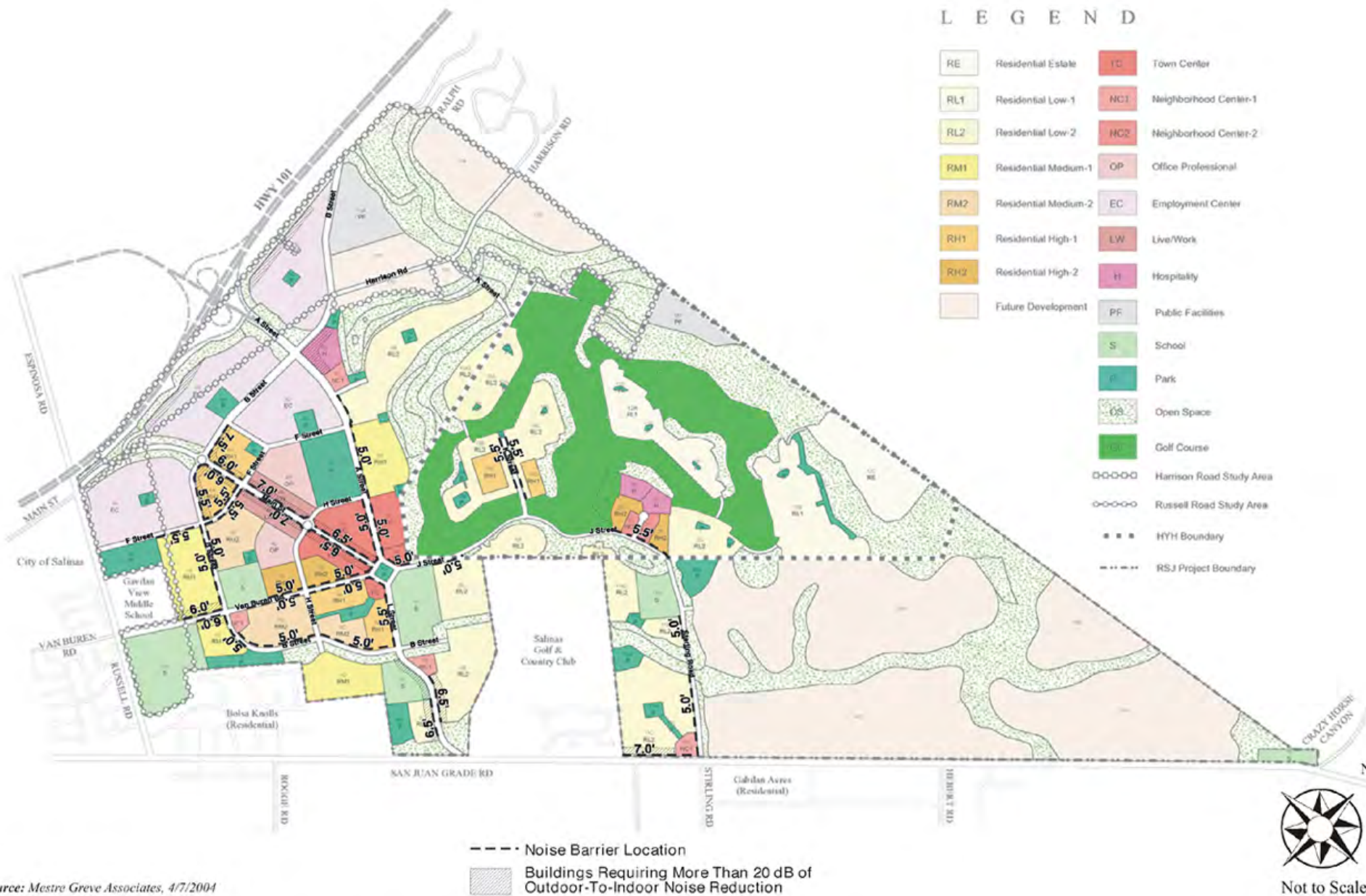
Noise Barrier Locations (Alternative 2)
